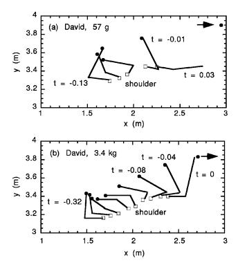
Fig. 3. Positions of the shoulder, upper arm, forearm, and thrown mass at 0.04-s time intervals. The (x,y) origin is a point at the bottom left corner of the video film. Time t=0 corresponds to the instant at which the mass was released.
