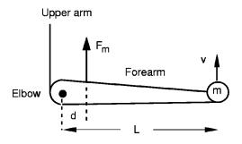
Fig. 8. The force F = mdv/dt acting on a mass *m* in the hand is determined by the muscle force  $F_m$  which exerts a torque  $\tau = F_m d$  about an axis through the elbow.
