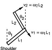
Fig. 4. Two segment model of throwing arm.
