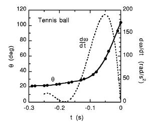
Fig. 9. Angular displacement,  $\theta$ , and acceleration,  $\alpha = d\omega/dt$ , of the forearm vs time when only the forearm is used to throw a tennis ball. The solid curve is sixth-order polynomial fitted to the experimental data (closed dots) to calculate the acceleration, assuming that  $\alpha = 0$  at t=0 (the time at which the ball was released).
