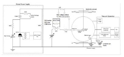
The experimental setup comprises of a pulsed high voltage power supply, a Langmuir probe on a linear stage and associated current measurement circuitry, a Helmholtz coil pair capable of producing a uniform field at the anode centre, a filament electron gun with extraction grid, and an orthodox set of vacuum apparatus
