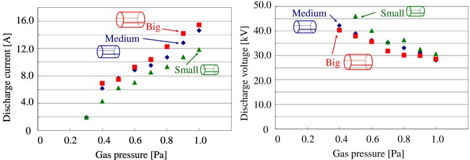
When the bigger cathode is used, the higher current flows and the discharge voltage becomes lower.
