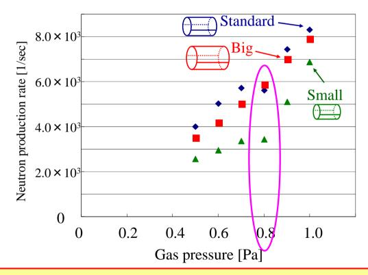
At 0.8Pa, bigger cathode has a good performance of neutron production rate and Neutron production rate of big cathode is 1.8 times of the small.
