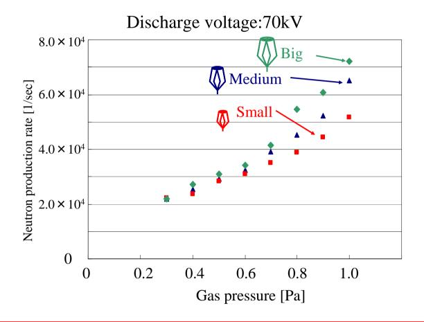
This graph shows that bigger cathode has a good performance of neutron production rate . When the big cathode is used, more ion beam is extracted from the ion source, and the Neutron production rate is increased.
