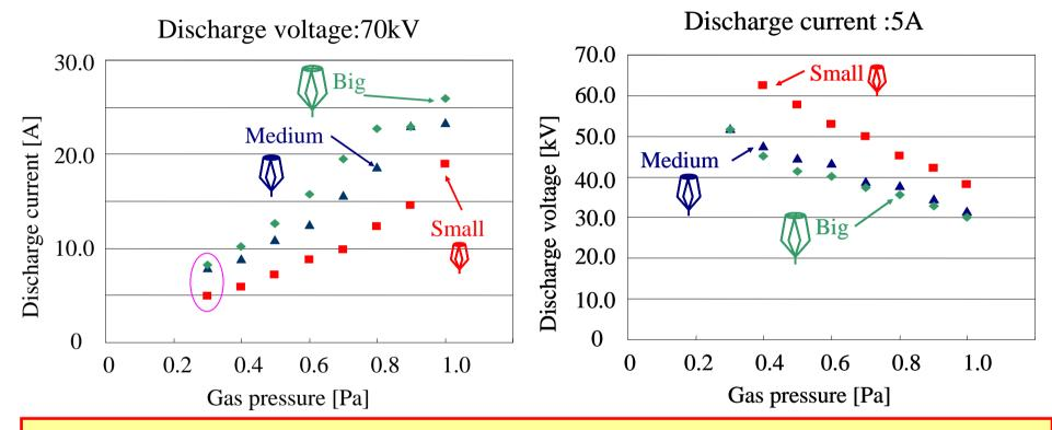
When the gas pressure becomes low, the discharge current is low and the voltage becomes high.
