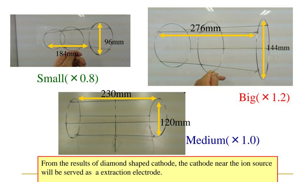
So, the cylindrical cathode is designed.
