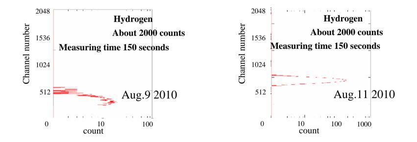
These figures are the noise signals that measured in another day. The energy level of the noise signal differs by the slight change of experiment condition. Therefore, that a noise occurs in 0.4Pa every time; cannot be concluded. Of course, this E-M noise is eliminated by doing everything possible.
