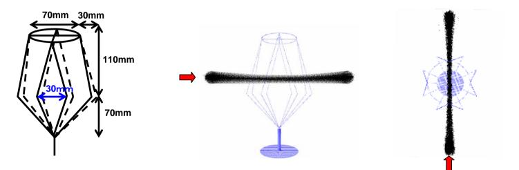
If the cathode is set closer to the ion source, the neutron production rate might be raised.
