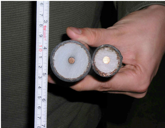
Photo showing current HV cable (right) and new HV cable (left)
