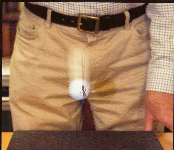
Position of golf ball at start of drop and after two bounces off a horizontal granite slab. The ball 'walked' its way to the left edge of the slab in this series of bounces.
