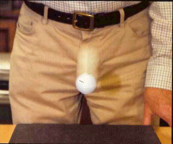
Position of golf ball at start of drop and after two bounces off a horizontal granite slab. The ball 'walked' its way to the left edge of the slab in this series of bounces.
