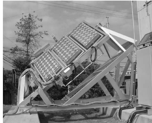
Figure 1: The concentrator PV system with flat Fresnel lens
