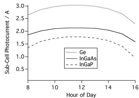
**Fig.9** Photocurrents generated in the respective InGaP, InGaAs and Ge sub-cells.
