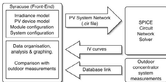
**Fig.2.** Schematic diagram showing how the Syracuse front end links with the SPICE circuit network solver and the outdoor measurement database.
