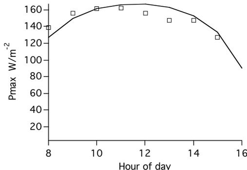
**Fig. 11** Comparison between the experimental power delivered by the module (squares) and that predicted by the model (line).
