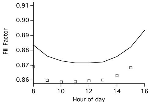
**Fig. 10** Comparison between the experimental fill-factor (squares) and calculated fill-factor (line.)
