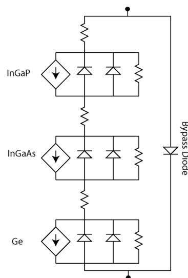
**Fig.4** Equivalent circuit for a single multi-junction cell packaged with a bypass diode into a receiver [7]
