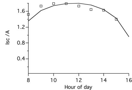
**Fig.8** Comparison between the measured (squares) and simulated (line) short-circuit current.
