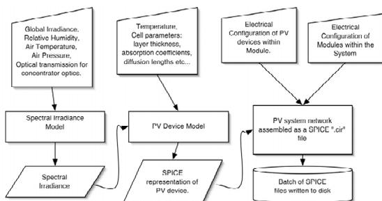
**Fig 3.** Process in the Syracuse front-end leading to the generation of SPICE netlist files. User inputs at the top and processes are represented by rectangles.
