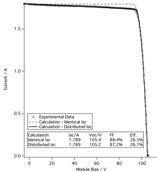
**Fig 5.** Experimental 400X module data and two simulated IV-curves, showing the effect of current mismatched cells.
