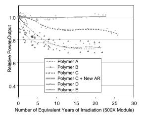
Fig. 5. Acceleration test by compound stress of simultaneous concentrated UV irradiation and water condensation.
