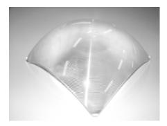
Fig. 2. 550X concentrator Fresnel lens made by injection molding. The size is 165 mm square.
