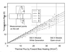
Fig. 7. Cell temperature relative to module temperature with given thermal flux
