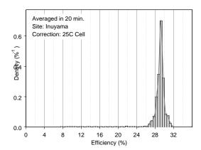
Fig. 7. Histogram of the corrected module efficiency in a clear summer day
