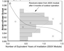
Fig. 4. Comparison between the acceleration test and outside exposure test
