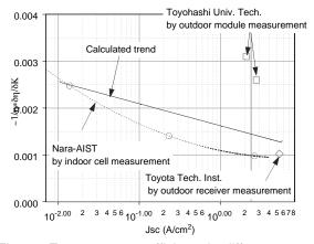
Fig. 6. Temperature coefficients in different concentration ratio by both indoor and outdoor measurements
