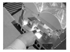
Fig. 8. Off-axis beam test : Thanks to the optical characteristics of the non-imaging Fresnel lens etc, fingers will not be burnt by off-axis beam
