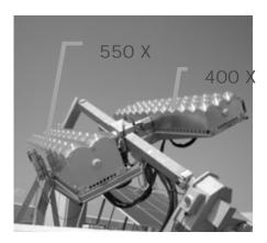
Fig. 1. 400X and 550X concentrator module on the same tracker in Toyohashi Site operated by Toyohashi University of Technology
