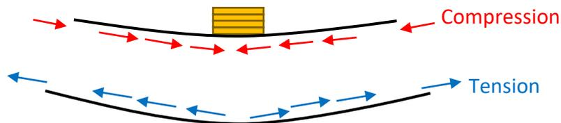
This means the particles in the top surface are in compression, they are pushed closer together. As the particles move closer together they begin to feel a push from the next particle. This balances the external compression and stops the particles moving any closer.
