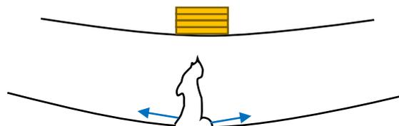
Eventually, when enough weights are added, the tension along the bottom edge of the plank is so great that the pull between neighbouring particles can no longer match it. The particles continue to move apart and the solid structure is broken - the plank cracks.
