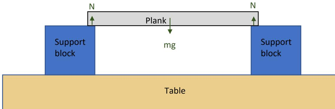
The support blocks provide a normal force upwards that balances the downwards weight force of the plank. It is in equilibrium (i.e. there is no unbalanced force and no movement).
