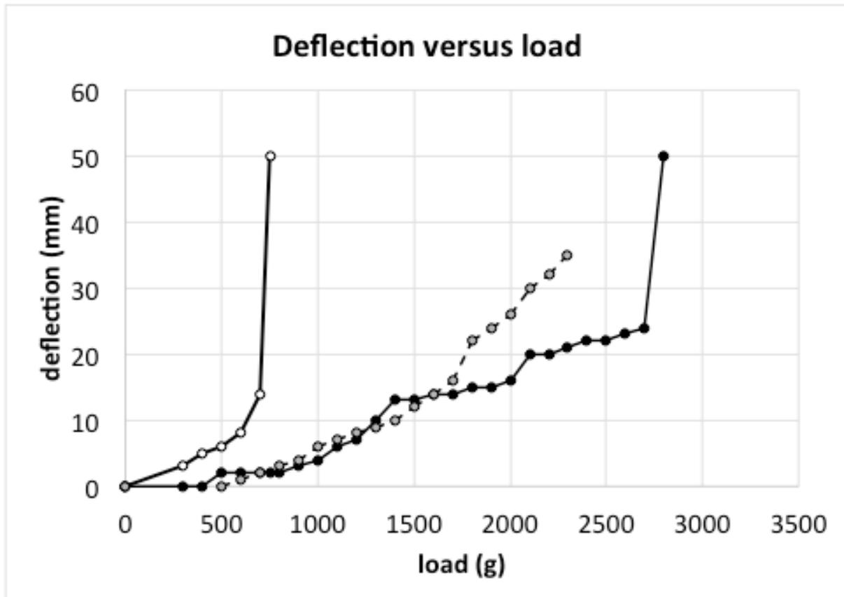
The graph shows the deflection of the polystyrene (vertical axis) when load (i.e. weights, horizontal axis) is applied to the centre of the polystyrene.
