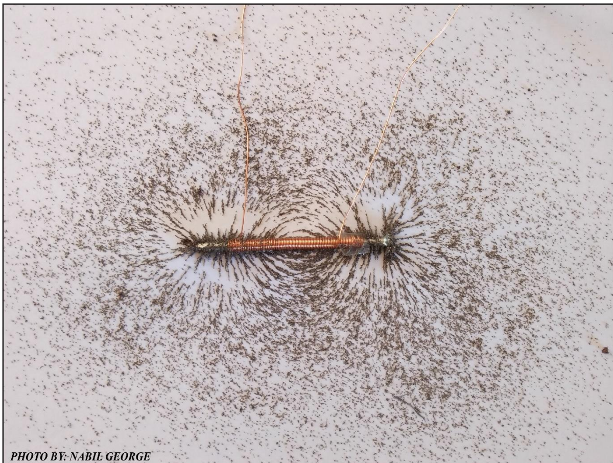
Figure 2: The iron filings around the electromagnet depicts the magnetic field lines.
