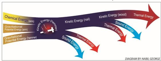
Mark on the 'Sankey' diagram above the actions of the arm, hammer, nail, and the wood.
