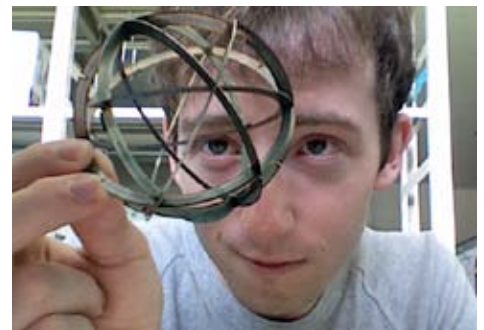
Looking at one of the gridded spherical cathodes used for IEC.
