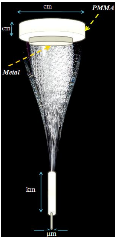
Figure 5 Fibre Drawing process
