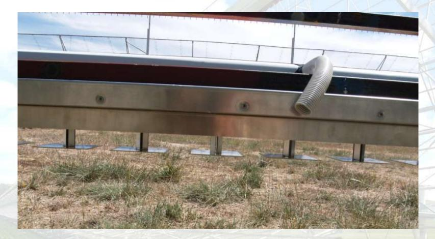
Analogue Beam-forming prototypes designed: Stage 1 combines the 8 elements of a module Stage 2 combines 6 modules, gives 4 outputs per bay
