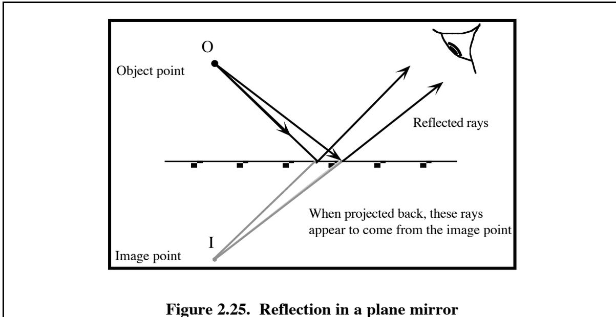
**Figure 2.25. Reflection in a plane mirror**
