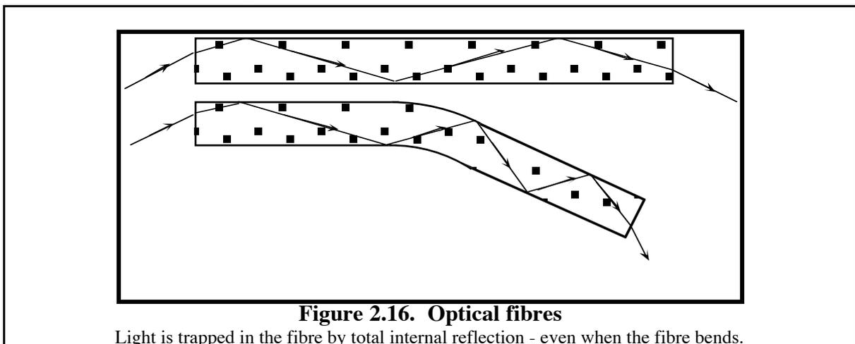
Optical fibres have many uses including data transmission, an alternative to sending electrical signals along conducting cables. The advantage of optical fibres here is that the capacity of the medium to carry information is vastly greater. Many different signals can be sent along the same fibre; in more technical terms, optical fibres have large bandwidths.
