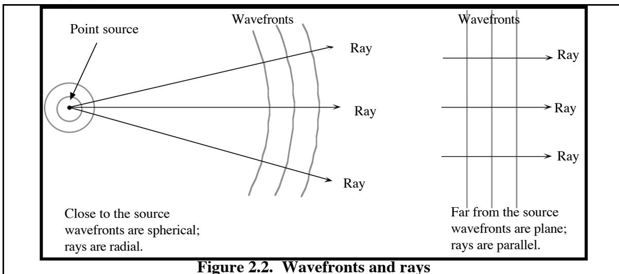
**Figure 2.2. Wavefronts and rays**
