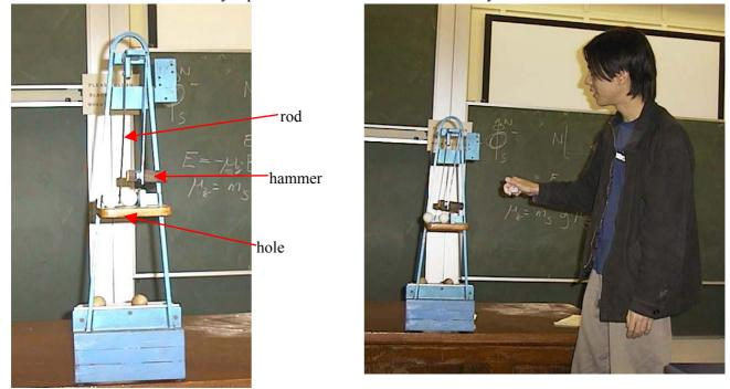
When the student releases the hammer it will swing back, striking the rod which holds the first ball in place over the hole, and knocking it into the second ball. The first ball drops directly down, the second follows a parabola.
