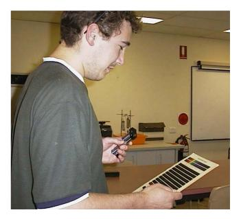
Students at the Australian Catholic University looking at the spectrum of fluorescent lights and using a chart of known spectra to identify the element (mercury) contained in the lights.
