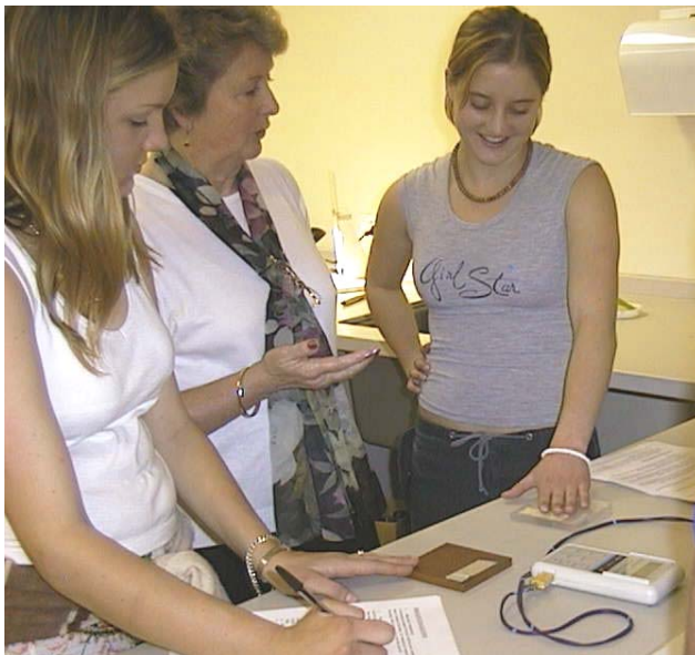
Students at the Australian Catholic University comparing the thermal conductivity of different materials.
