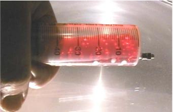
The syringe contains water and food colouring so that the bubbles are easier to see. The water boils, forming bubbles when the plunger is pulled causing a drop in pressure.
