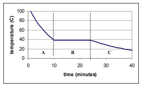
2. Heat can be added to a substance without causing the temperature of the substance to rise.
