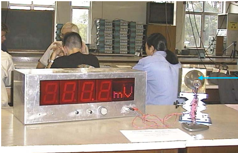
Thermopile detector in front of the Leslie cube in a workshop tutorial at the University of New South Wales
