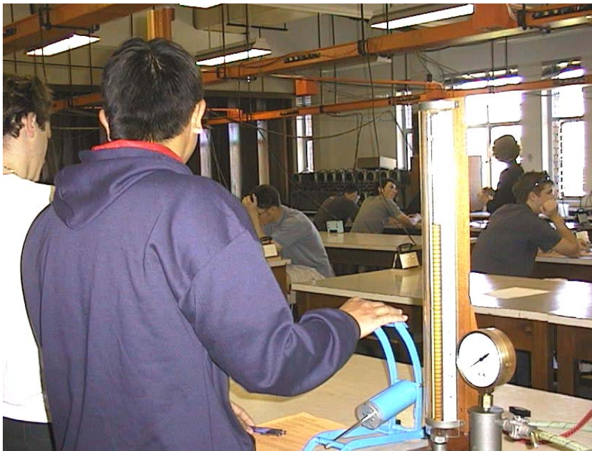
Students at the University of New South Wales using the Boyle's law apparatus.
