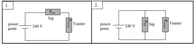
The toaster has an operating resistance of 30  $\Omega$  and the electric jug has a resistance of 40  $\Omega$ . **a.** Calculate the total resistance of each circuit.
