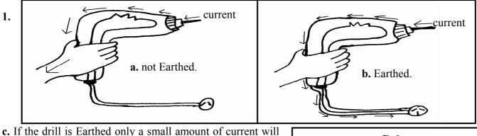
flow through Brian, especially if he is wearing rubber soled boots. The Earth connection provides a path of very low resistance for the current. If the drill is not Earthed the path of least resistance from the power cable through the drill and to Earth is via Brian. Brian will probably be burnt, receive a shock, and may even be electrocuted.
