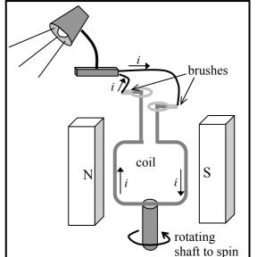
**c.** According to Lenz's law the current flows to counteract the change in magnetic flux. As the coil turns from parallel to the field to perpendicular the magnetic flux increases. As it continues to turn the magnetic flux decreases again. While the flux is increasing the current flows in one direction and while the flux decreases the current flows the opposite way. Hence an alternating current is produced.
