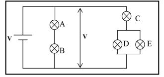
Hence the resistance of this arm is 3/2 times that of a single globe. Globe C will have a potential difference of 2/3 of the voltage V, and D and E will each have 1/3 V. Brightness increases with power which goes like the  $V^2$ , so we can rank the brightness by ranking the voltages. Hence the order of brightness will be C  $\rightarrow$  A & B  $\rightarrow$  D & E (brightest to dimmest).
