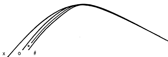
Figure 4—Intensity spectra for cubic and spherical sources with the electron density falling away from the centre of the sphere. Curves labelled x, o, and * are spherical sources with m=2, 1 and 0 respectively; # is a cubic model. The value of a is 3 for each curve.
