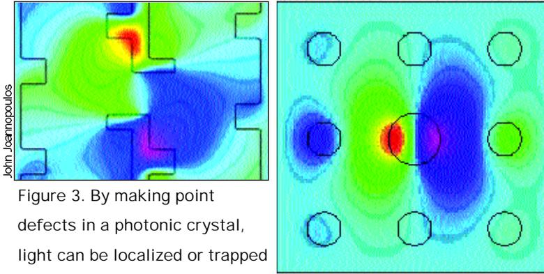
Figure 3. By making point defects in a photonic crystal, light can be localized or trapped in the defect. Since the properties of defects can be finely tuned, such crystals make very sharp filters.
