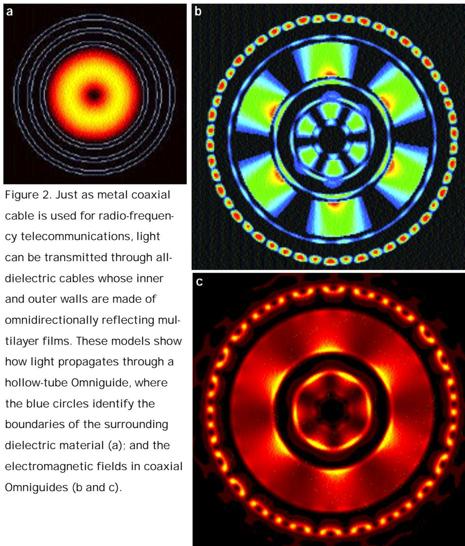
Figure 2. Just as metal coaxial cable is used for radio-frequency telecommunications, light can be transmitted through all-dielectric cables whose inner and outer walls are made of omnidirectionally reflecting multilayer films. These models show how light propagates through a hollow-tube Omniguide, where the blue circles identify the boundaries of the surrounding dielectric material (a); and the electromagnetic fields in coaxial Omniguides (b and c).
