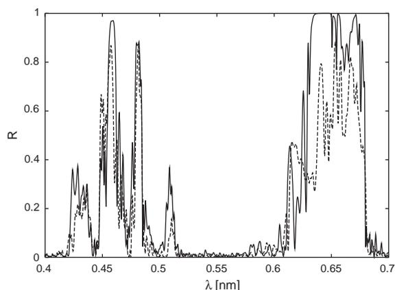
Fig. 2.  $E$  (solid curve) and  $H$  (dashed curve) polarization normal incidence reflectance for an 88 layer stack of gratings having the geometric structure of the sea mouse spine of Fig. 1.
