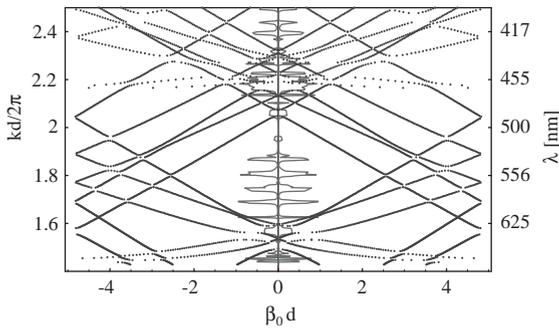
Fig. 4. Band diagram for  $E$  polarization and normal incidence on the long side of the unit cell. On the abscissa we represent the crystal momentum  $\mathbf{k}_0 = (0, \beta_0)$  for normal incidence. The values of  $\beta_0$  corresponding to each  $k = 2\pi/\lambda$ , are the eigenvalues of a scattering matrix [6].
