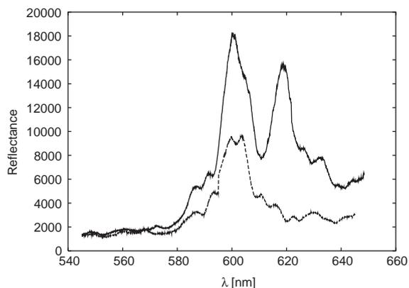
Fig. 3. Microreflectance measurements on a green-gold sea mouse hair.
