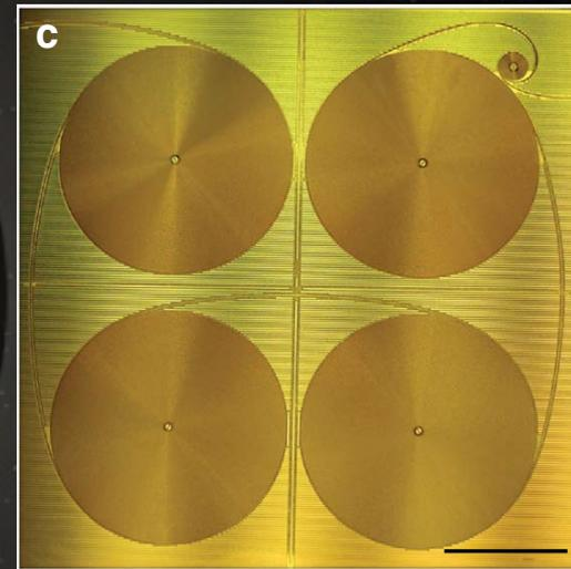
larger. Here we demonstrate a monolithic waveguide as long as 27 m (39 m optical path length), and featuring broadband loss rate values of  $(0.08 \pm 0.01) \text{ dB m}^{-1}$  measured over 7 m by optical
