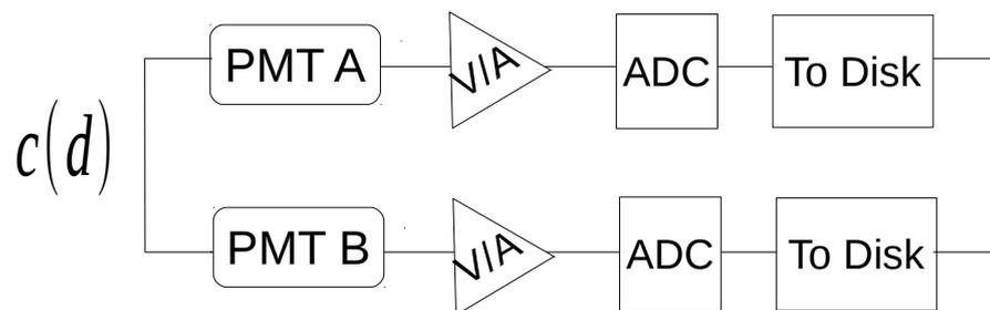
$$c_m = c(d) G_{pmt A} G_{pmt B} G_{pre-amp}^2 G_{ADC}^2$$
