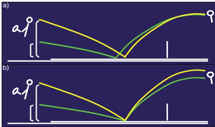
Figure 3. In a) variation of the height for return according to the depth of the bounce, and b) the same variation resulting from the variation of the impact height in service.
