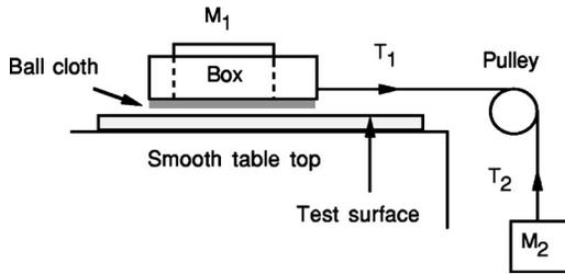
Fig. 1. Arrangement used to measure the coefficient of friction (COF) at low sliding speeds.
