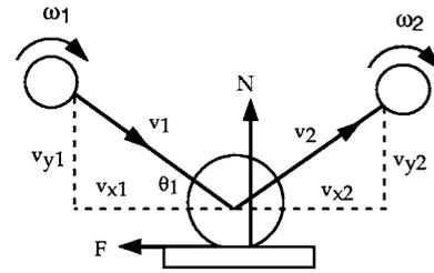
Fig. 2. Oblique impact of a ball on a horizontal surface.  $F$  is the friction force and  $N$  is the normal reaction force.  $N$  does not necessarily act through the center of the ball, and  $F$  is not necessarily equal to  $\mu N$ .
