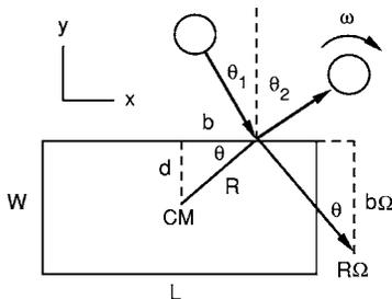
Fig. 2. Plan view of the gear effect experiment showing the positive directions for  $x$ ,  $y$ ,  $\omega$ ,  $\theta_1$ , and  $\theta_2$ . The gear effect is dominant at large  $b$ , large  $d$ , and small  $\theta_1$ , resulting in a counter-clockwise spin of the ball ( $\omega < 0$ ) when the block rotates clockwise ( $\Omega > 0$ ).
