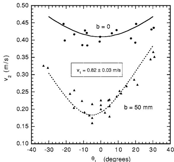
Fig. 5. Experimental values of the rebound speed  $v_2$  versus the angle of incidence  $\theta_1$  for a golf ball impacting a 210 g wood block with  $b=0$  (dots) and  $b=50$  mm (triangles). Also shown are the theoretical estimates derived in the Appendix for the same parameters as those indicated in Fig. 3.
