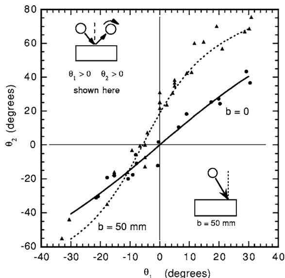
Fig. 4. Experimental values of the rebound angle  $\theta_2$  versus the angle of incidence  $\theta_1$  for a golf ball impacting a 210 g wood block with impact parameter  $b=0$  (dots) and  $b=50$  mm (triangles). Also shown are the theoretical estimates derived in the Appendix for the same parameters as those in Fig. 3.
