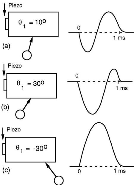
Fig. 6. Output signals from a piezo disk attached to one end of the block. A positive (negative) output indicates acceleration of the block to the left (right). The dashed line in each trace is the zero acceleration level. In each case, the ball was incident without spin and commenced sliding along the block. Reversal of the signal indicates a grip phase followed by a reversal in the sliding direction. The grip phase commenced earlier in (a) than in (b), resulting in a smaller ball spin.
