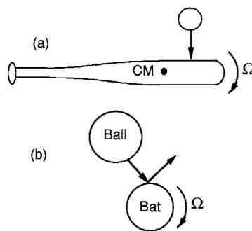
Fig. 7. A ball impacting on a baseball bat can result in bat rotation about two different axes, as shown in (a) and (b).
