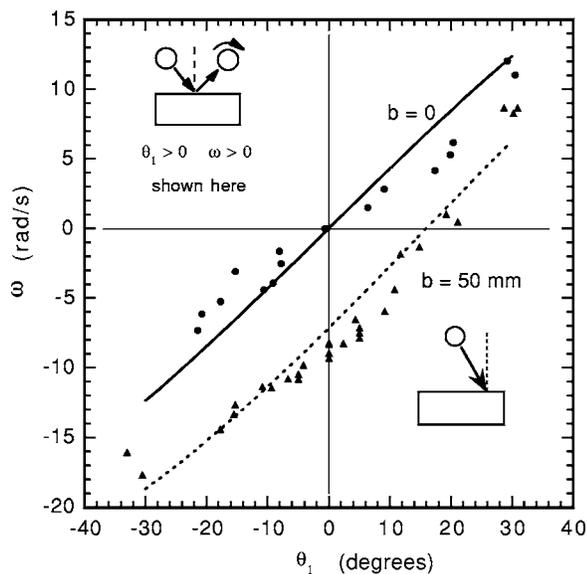
Fig. 3. Experimental values of the ball spin,  $\omega$  versus the angle of incidence  $\theta_1$  for a golf ball impacting a 210 g wood block with impact parameter  $b=0$  (dots) and  $b=50$  mm (triangles). Also shown are the theoretical estimates based on Eq. (A15) with  $e_x=0$  and  $e=0.83$  for  $b=0$  and  $e=0.89$  for  $b=50$  mm.
