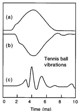
Fig. 6. Results for a tennis ball showing (a) the output of the 50 mm diam piezo, (b) the output of a small piezo (at 50 mV/div) mounted on the ball at a point 30° away from the contact point, and (c) the output of the small piezo (at 10 mV/div) mounted on the top of the ball, i.e., at a point 180° away from the contact point.
