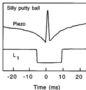
Fig. 4. The force wave form observed with a silly putty ball, and the  $L_1$  laser beam signal observed when  $L_1$  is located 11 mm above the piezo surface. The ball had a mass of 12.9 gm and a diameter of 29 mm. The ball blocks the beam 5 ms before it hits the piezo and unblocks the beam 7 ms after it leaves the surface.
