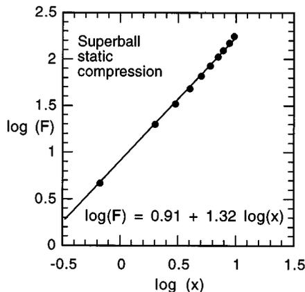
Fig. 8. The static compression curve for a superball [Fig. 5(b)] plotted on a log–log scale.
