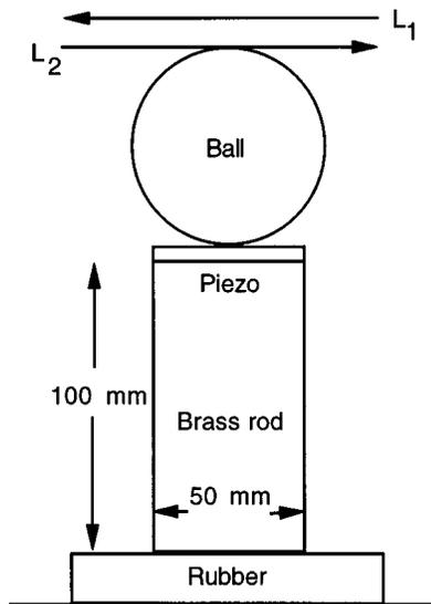
Fig. 1. The arrangement used to measure the ball speed and force wave forms. Here  $L_1$  and  $L_2$  are horizontal laser beams separated vertically by 10 mm.
