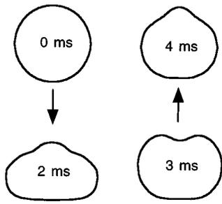
Fig. 7. Cross section of a tennis ball during a 100 mph collision with a concrete slab. The ball impacts at  $t=0$  and rebounds at  $t\sim 4$  ms.
