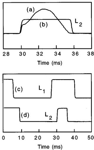
Fig. 3. The force wave form (a), and the laser beam signals (b), (c), (d) for a tennis ball when the lower beam  $L_2$  just grazes the top of the ball, as shown in Fig. 1.  $L_2$  is unblocked during the impact and for 0.4 ms after the impact. Trace (b) is an expanded version of trace (d).
