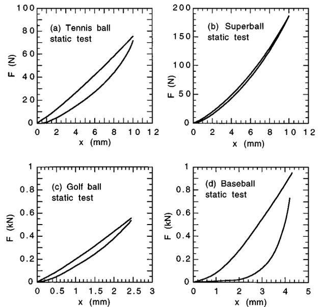
Fig. 5. Static hysteresis curves for four different balls showing the applied force  $F$  versus the compression,  $x$ , when the ball is compressed and then decompressed between parallel metal plates.
