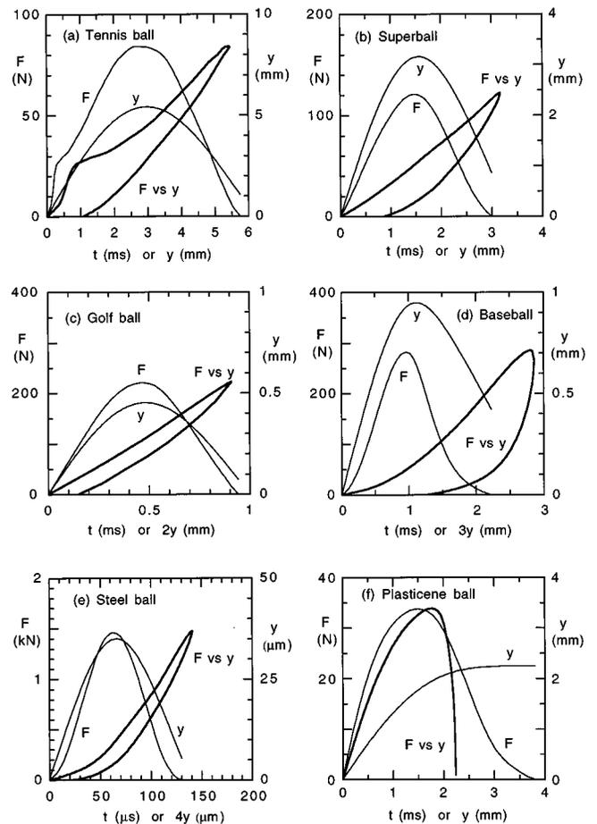
Fig. 2.  $F$  and  $y$  vs time for six different balls, together with the corresponding  $F$  vs  $y$  dynamic hysteresis curves, where  $y$  is the displacement of the center of mass. The ball speeds are listed in Table I.
