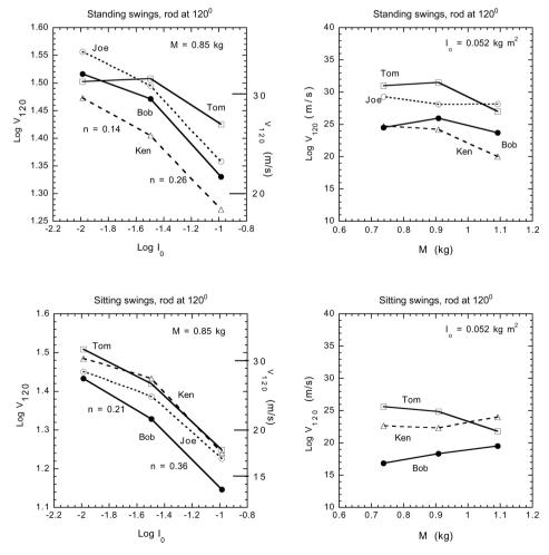
Figure 3.  $V_{120}$  results for both standing and seated positions. For the constant mass rods, log  $V_{120}$  is plotted on the left vertical scale with a translation to  $V_{120}$  on the right vertical scale.
