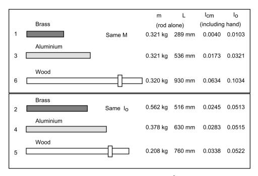
Figure 1. Rods used in the experiment. The moments of inertia  $I_{cm}$  and  $I_o$  (units kg·m<sup>2</sup>) refer to axes through the centre of mass and the handle (left) end, respectively.
