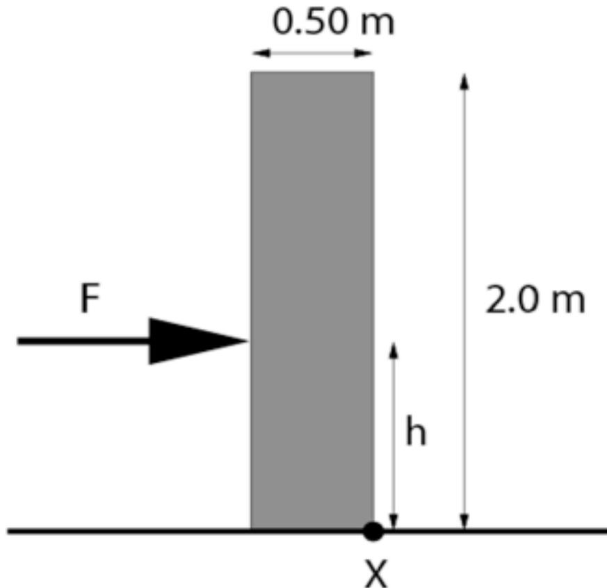
If the block is pushed too near to the top, it will tip over instead of sliding. It will try to rotate about the front corner of the block (labelled X in the diagram).
