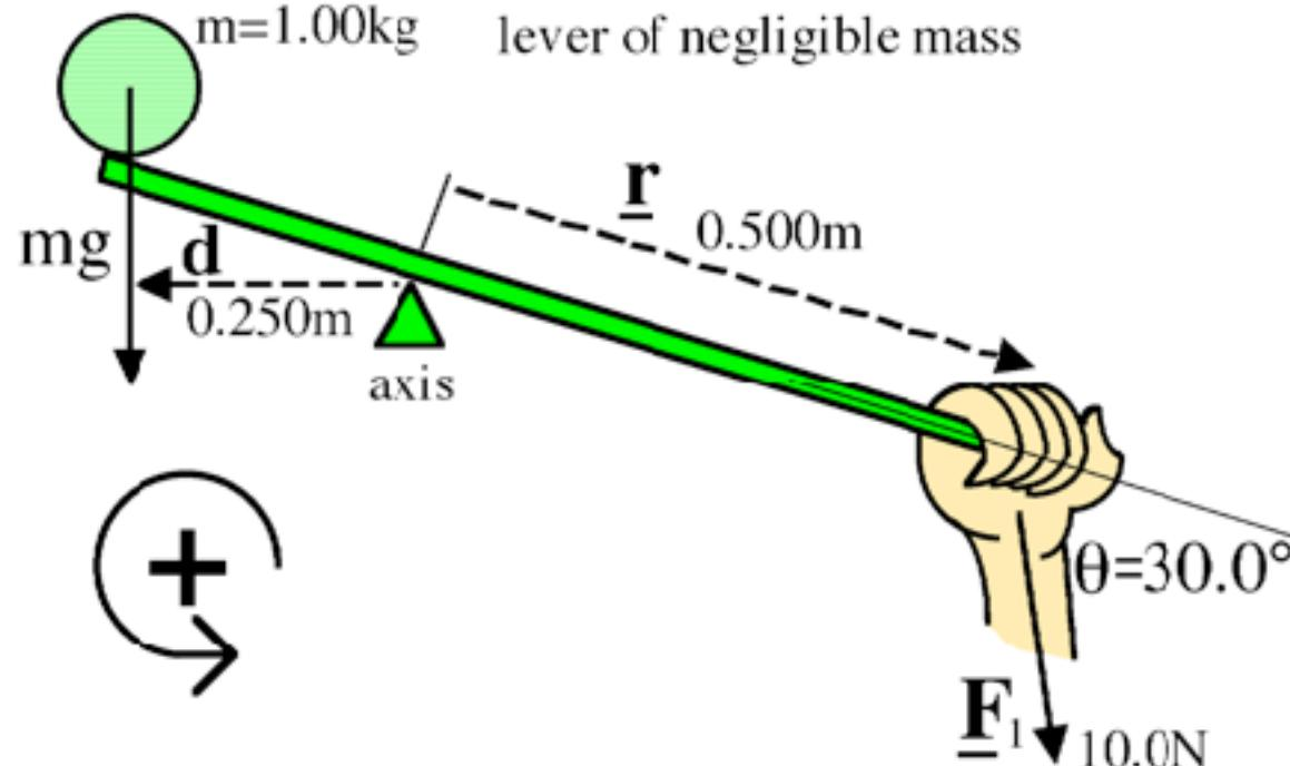
$$\text{torque 1; } \underline{\tau}_1 = -rF_1 \sin\theta = -0.5 \times 10 \times \sin 30 = -2.50 \text{ Nm}$$
