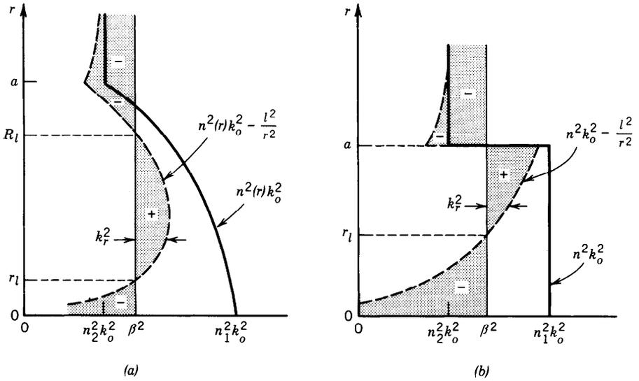
**Figure 8.2-5** Dependence of  $n^2(r)k_o^2$ ,  $n^2(r)k_o^2 - l^2/r^2$ , and  $k_r^2 = n^2(r)k_o^2 - l^2/r^2 - \beta^2$  on the position  $r$ . At any  $r$ ,  $k_r^2$  is the width of the shaded area with the + and - signs denoting positive and negative  $k_r^2$ . (a) Graded-index fiber;  $k_r^2$  is positive in the region  $r_l < r < R_l$ . (b) Step-index fiber;  $k_r^2$  is positive in the region  $r_l < r < a$ .
