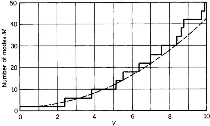
**Figure 8.1-8** Total number of modes  $M$  versus the fiber parameter  $V = 2\pi(a/\lambda_0)NA$ . Included in the count are two helical polarities for each mode with  $l > 0$  and two polarizations per mode. For  $V < 2.405$ , there is only one mode, the fundamental  $LP_{01}$  mode with two polarizations. The dashed curve is the relation  $M = 4V^2/\pi^2 + 2$ , which provides an approximate formula for the number of modes when  $V \gg 1$ .
