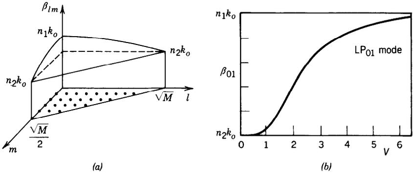
**Figure 8.1-10** (a) Approximate propagation constants  $\beta_{lm}$  of the modes of a fiber with large  $V$  parameter as functions of the mode indices  $l$  and  $m$ . (b) Exact propagation constant  $\beta_{01}$  of the fundamental  $LP_{01}$  modes as a function of the  $V$  parameter. For  $V \gg 1$ ,  $\beta_{01} \approx n_1 k_o$ .
