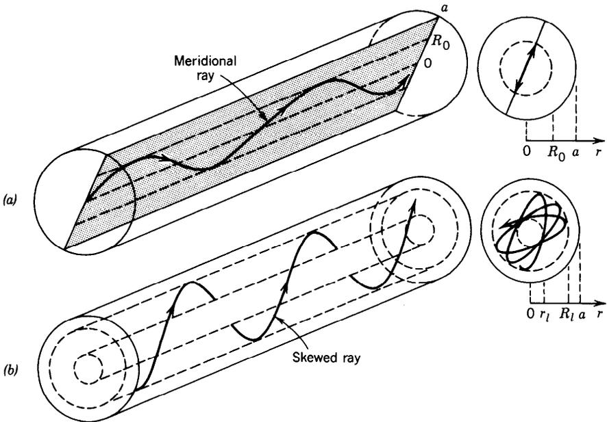
**Figure 8.2-3** Guided rays in the core of a graded-index fiber. (a) A meridional ray confined to a meridional plane inside a cylinder of radius  $R_0$ . (b) A skewed ray follows a helical trajectory confined within two cylindrical shells of radii  $r_1$  and  $R_1$ .
