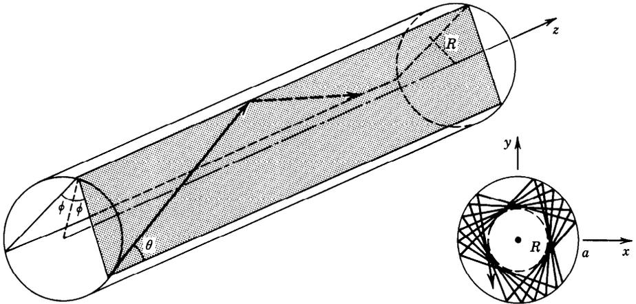
**Figure 8.1-2** A skewed ray lies in a plane offset from the fiber axis by a distance  $R$ . The ray is identified by the angles  $\theta$  and  $\phi$ . It follows a helical trajectory confined within a cylindrical shell of radii  $R$  and  $a$ . The projection of the ray on the transverse plane is a regular polygon that is not necessarily closed.
