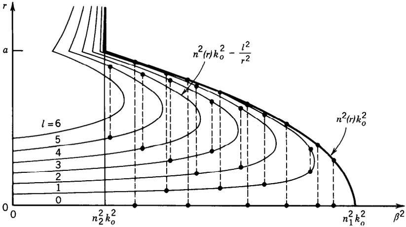
**Figure 8.2-6** The propagation constants and confinement regions of the fiber modes. Each curve corresponds to an index  $l$ . In this plot  $l = 0, 1, \dots, 6$ . Each mode (representing a certain value of  $m$ ) is marked schematically by two dots connected by a dashed vertical line. The ordinates of the dots mark the radii  $r_1$  and  $R_1$  of the cylindrical shell within which the mode is confined. Values on the abscissa are the squared propagation constants  $\beta^2$  of the mode.
