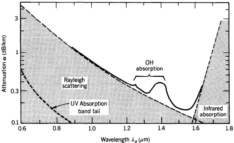
**Figure 8.3-2** Dependence of the attenuation coefficient  $\alpha$  of silica glass on the wavelength  $\lambda_o$ . There is a local minimum at  $1.3 \mu\text{m}$  ( $\alpha \approx 0.3 \text{ dB/km}$ ) and an absolute minimum at  $1.55 \mu\text{m}$  ( $\alpha \approx 0.16 \text{ dB/km}$ ).
