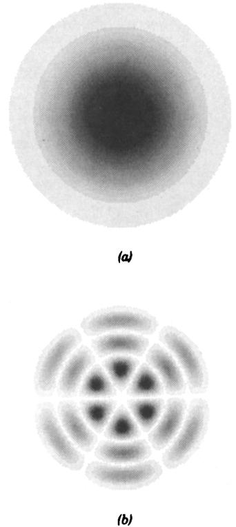
**Figure 8.1-7** Distributions of the intensity of the (a)  $LP_{01}$  and (b)  $LP_{34}$  modes in the transverse plane, assuming an azimuthal  $\cos l\phi$  dependence. The fundamental  $LP_{01}$  mode has a distribution similar to that of the Gaussian beam discussed in Chap. 3.
