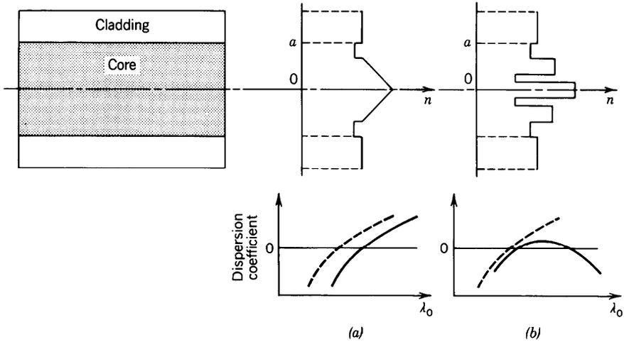
**Figure 8.3-6** Refractive-index profiles and schematic wavelength dependences of the material dispersion coefficient (dashed curves) and the combined material and waveguide dispersion coefficients (solid curves) for (a) dispersion-shifted and (b) dispersion-flattened fibers.
