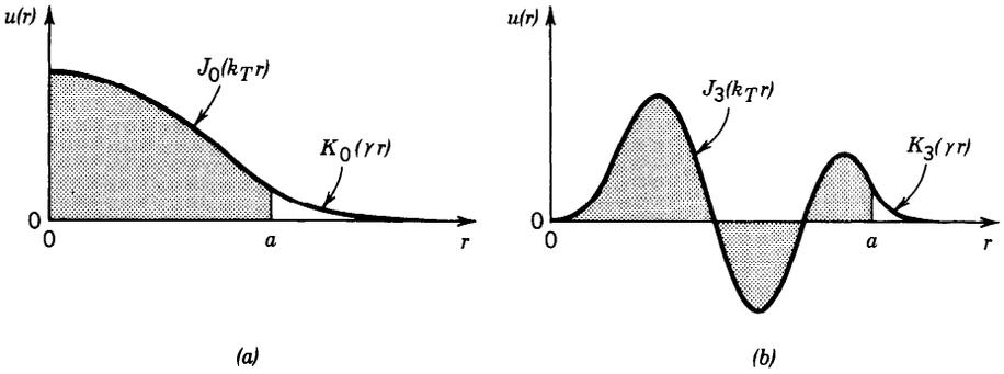
**Figure 8.1-5** Examples of the radial distribution  $u(r)$  given by (8.1-9) for (a)  $l = 0$  and (b)  $l = 3$ . The shaded areas represent the fiber core and the unshaded areas the cladding. The parameters  $k_T$  and  $\gamma$  and the two proportionality constants in (8.1-9) have been selected such that  $u(r)$  is continuous and has a continuous derivative at  $r = a$ . Larger values of  $k_T$  and  $\gamma$  lead to a greater number of oscillations in  $u(r)$ .
