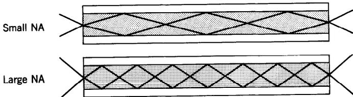
**Figure 8.1-3** (a) The acceptance angle  $\theta_a$  of a fiber. Rays within the acceptance cone are guided by total internal reflection. The numerical aperture  $NA = \sin \theta_a$ . (b) The light-gathering capacity of a large NA fiber is greater than that of a small NA fiber. The angles  $\theta_a$  and  $\theta_c$  are typically quite small; they are exaggerated here for clarity.
