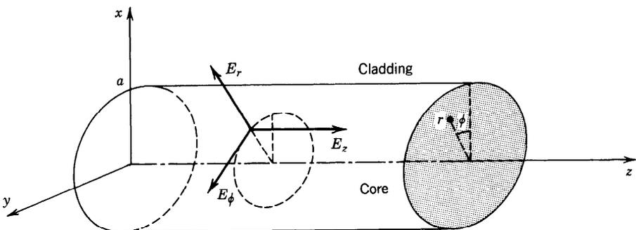
Figure 8.1-4 Cylindrical coordinate system.
