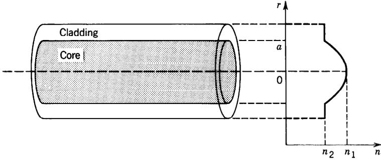
**Figure 8.2-1** Geometry and refractive-index profile of a graded-index fiber.
