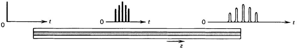
Figure 8.3-4 Pulse spreading caused by modal dispersion.
