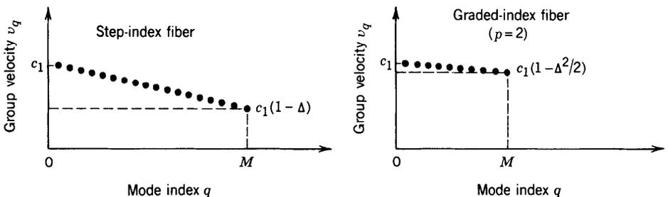
**Figure 8.2-8** Group velocities  $v_q$  of the modes of a step-index fiber ( $p = \infty$ ) and an optimal graded-index fiber ( $p = 2$ ).
