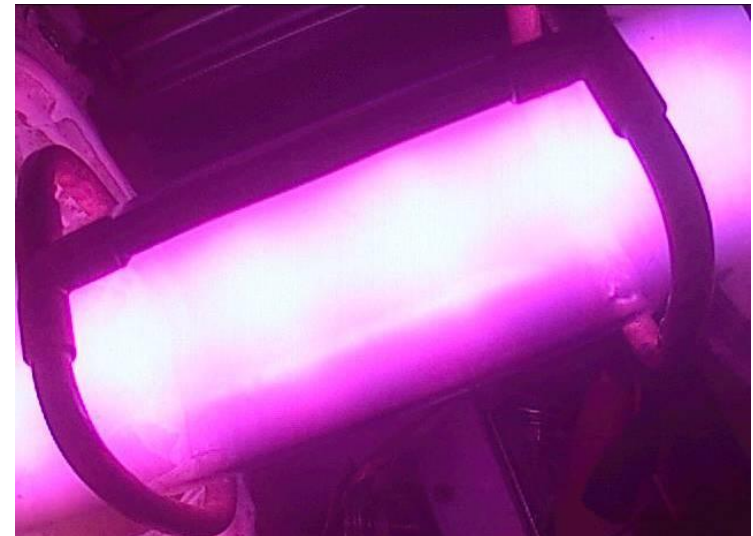
Hydrogen helicon plasma 1mTorr, 500 W, 500G
