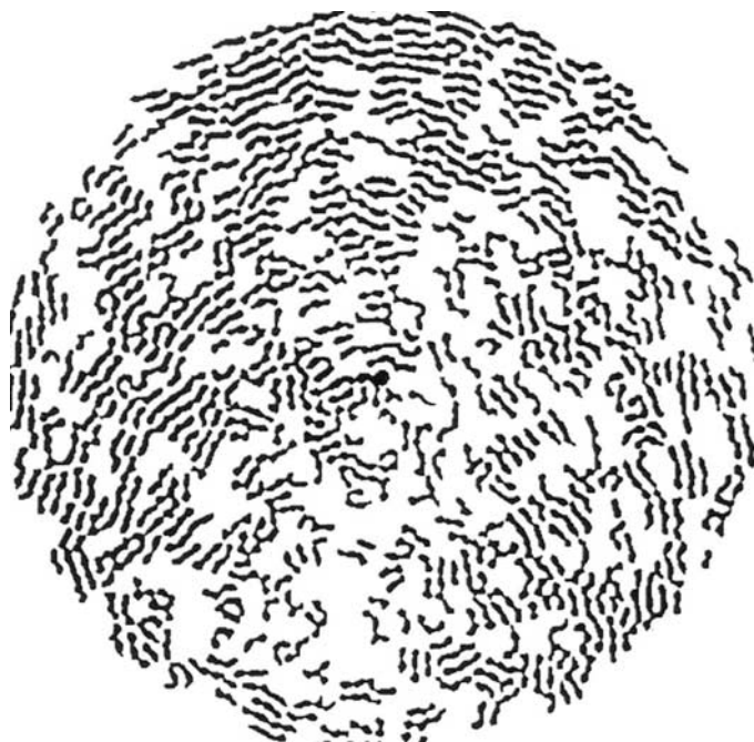
FIG. 19. Filtered pattern of soot particle structure. 83
