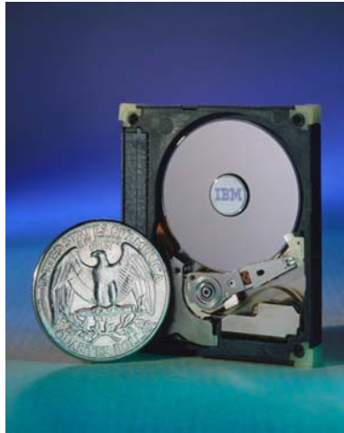
Fig. 7. IBM's ``quarter dollar'' 1 GB Microdrive.
