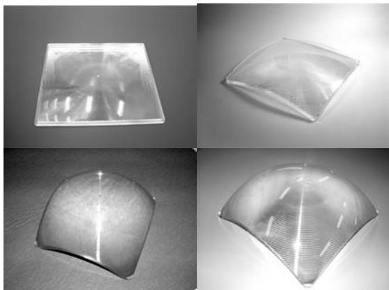
**Figure 5:** Generations of injection-molded Fresnel lenses
