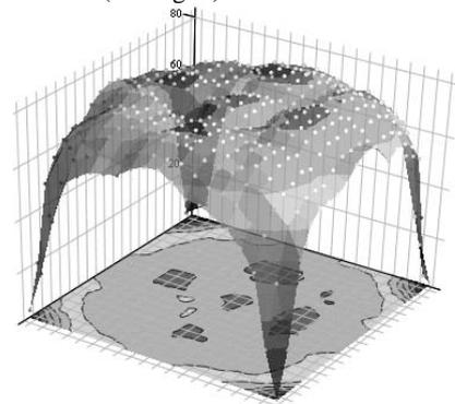
**Figure 6:** Distribution of 140 mm square 400 X Fresnel lens optical efficiency made by injection molding **before improvement**
