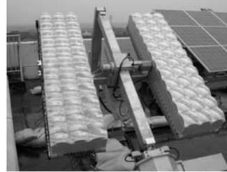
**Figure 11:** Field test in Toyohashi site, Rooftop of the building and relatively strong wind, 5 km North from sea
