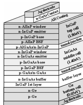
**Figure 3** Structure of the 3J concentrator cell
