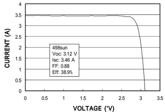
**Figure 2:** I-V curve of the 3J cell at 498 sun irradiation
