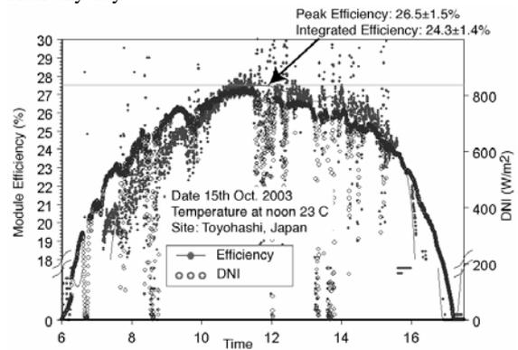
**Figure 13:** Power generation in a course of the day – sunny day with thin clouds
