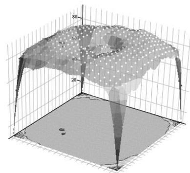
**Figure 7:** Distribution of 140 mm square 400 X Fresnel lens optical efficiency made by injection molding **after improvement**
