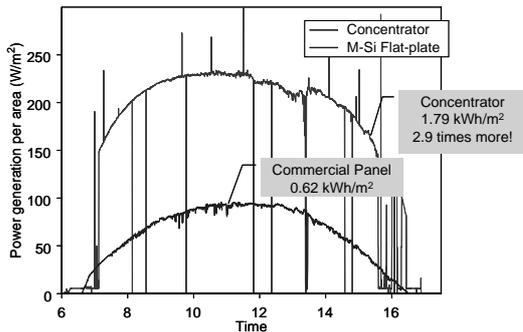
**Figure 14:** Comparison to a commercial flat-plate crystalline silicon module
