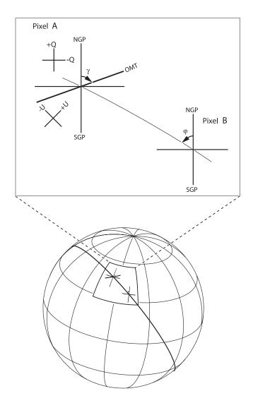
Fig. 1.—Geometry for Stokes Q and U parameters. WMAP measures polarization by differencing two orthogonal polarization channels, then solving for Q and U as the spacecraft compound spin projects the OMT onto the sky at different angles  $\gamma$  relative to the Galactic meridians. All analysis uses coordinate-independent quantities Q' and U' defined with respect to the great circle connecting a pair of pixels (see text).
