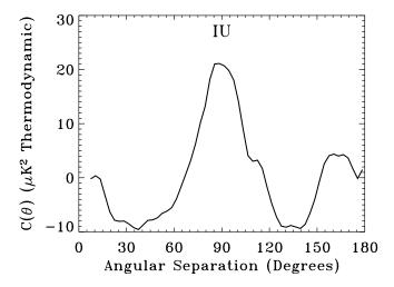
Fig. 3.—Angular templates for potential systematic errors caused by bandpass mismatch between the two radiometers in each DA. We fit this template to the correlation functions from each DA to detect or limit systematic errors related to bandpass mismatch in the main beam. The effect is significant only in the K and Ka bands, which have the brightest unpolarized foregrounds.
