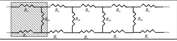
If  $R_o = R_i = R$ , then the resistance of the single section of membrane shown shaded in the diagram is  $2R + R_i = R_i = R_i$  $R_m$ . As the circuit is of effectively infinite length, the rest of the membrane to the right has a resistance effectively the same as the total resistance,  $R_T$ . This  $R_T$  is in parallel with the membrane resistance,  $R_m$ , so
