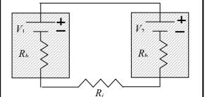
c. If Brent has connected the batteries together correctly the current which flows will be the total emf divided by the total resistance (Ohm's law) :
