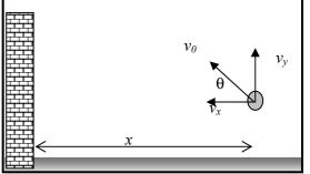
**a.** The ball is x = 10 m away from the wall to begin with. The time taken for the ball to reach the wall is  $t = x/v = x/(v_o \cos\theta) = 10$  m / (15 m.s<sup>-1</sup> cos 40°) = 0.87 s.
