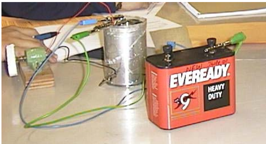
Large capacitor with battery and motor.
