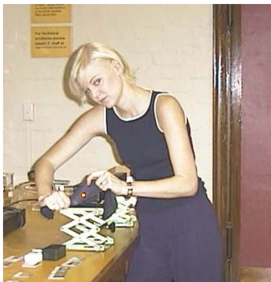
A piece of panty-hose material is used to make a diffraction pattern.
