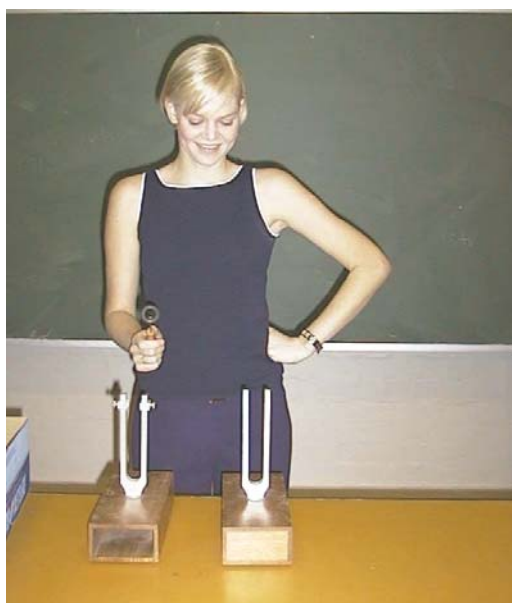
When the two tuning forks have similar frequencies beats can be heard.
