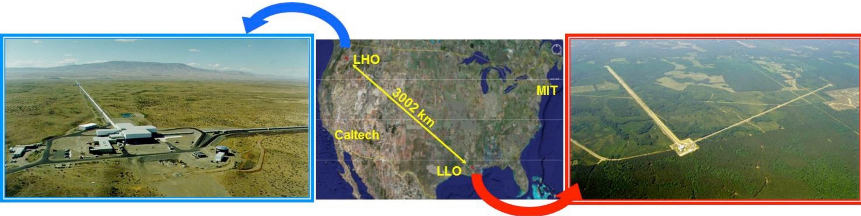
*The LIGO “observatory” is made up of two identical and widely separated interferometers situated in sparsely populated, out-of-the-way places: LIGO Hanford in southeastern Washington State, and LIGO Livingston, 3002 km away near Baton Rouge, Louisiana. Each arm is 4 km long.*
