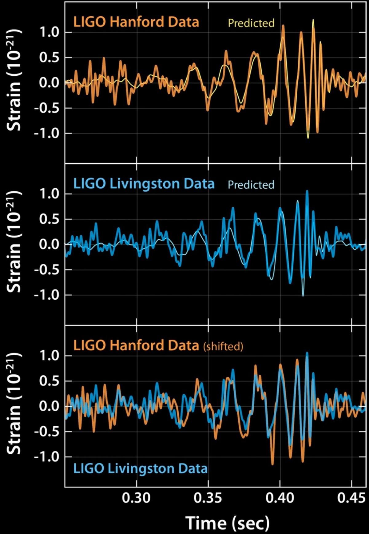
Over 0.2 s, the signal increases in frequency and amplitude in about 8 cycles, from 35 to 150 Hz (the “chirp”). The most plausible explanation for this signal is the inspiral of two orbiting masses due to gravitational wave emission.
