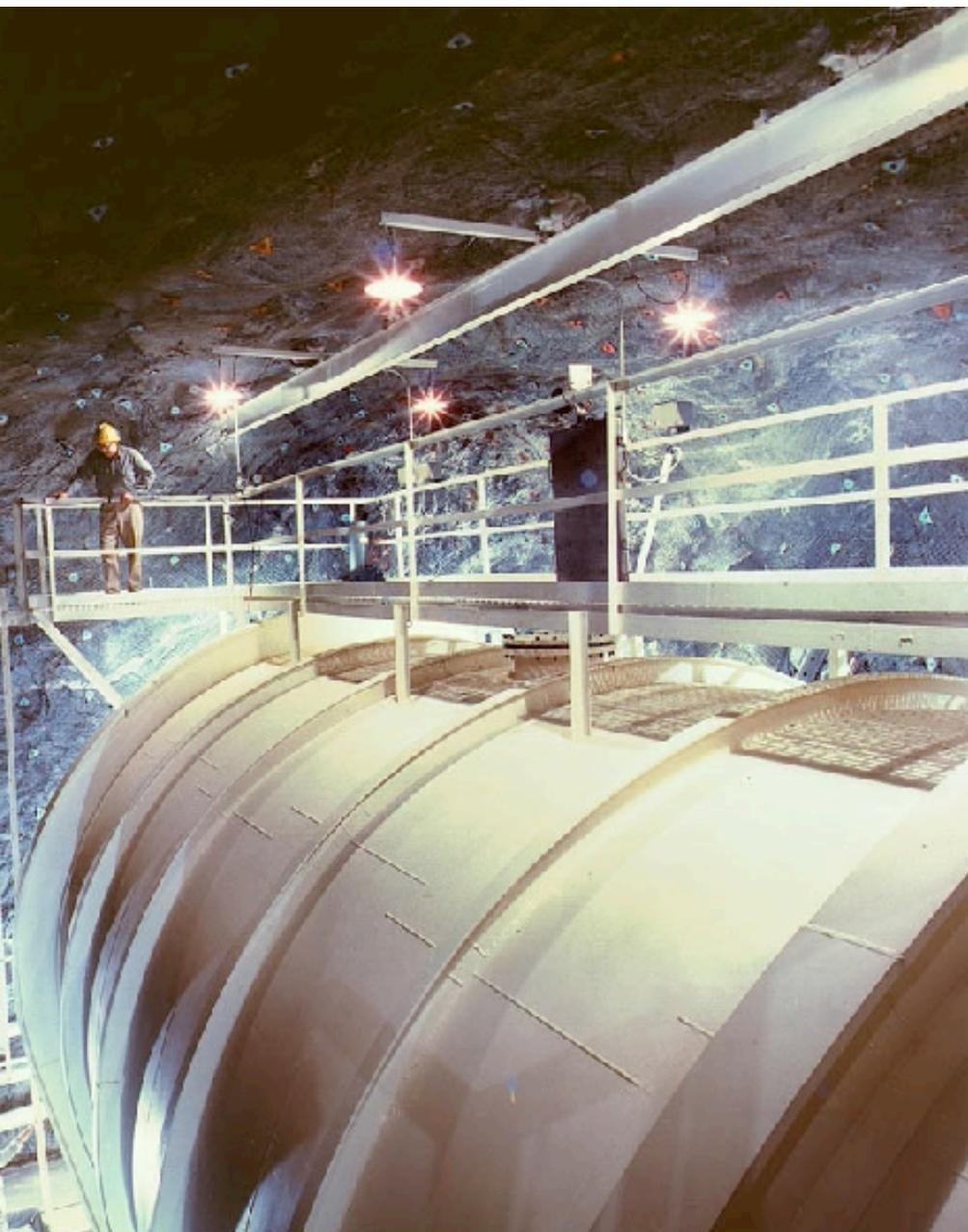
Raymond Davis built the first neutrino detector in the 1960s. The detector consisted of 400,000 litres of cleaning fluid (C<sub>2</sub>Cl<sub>4</sub>) one mile underground in an old mine.
