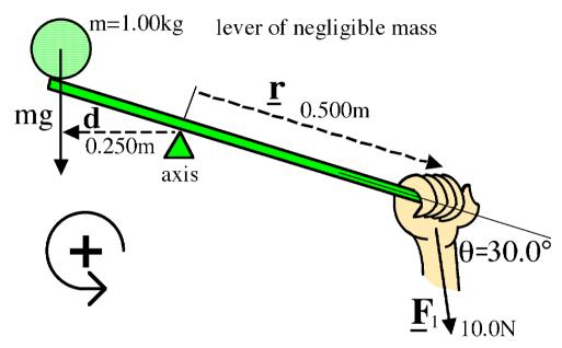
torque 1;  $\underline{\tau}_1 = -rF_1 \sin\theta = -0.5 \times 10 \times \sin 30 = -2.50 \text{ Nm}$
