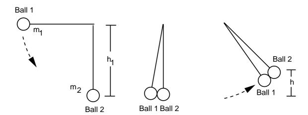
(a) The mechanical energy of ball 1 must be the same at the top of its swing and at the bottom where it is about to strike ball 2. We choose to set the potential energy of ball 1 to be zero when it is at the position of ball 2. Ball 1 has zero kinetic energy at the top because it is at rest initially.
