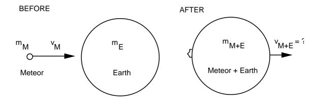
We use the fact that the total momentum of the Earth+Meteor system is conserved i.e. the same before and after the impact. This is an inelastic collision.
