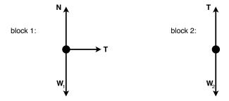
Because the blocks are linked by the string, the tension is the same for both blocks, and the acceleration is the same for both blocks.
