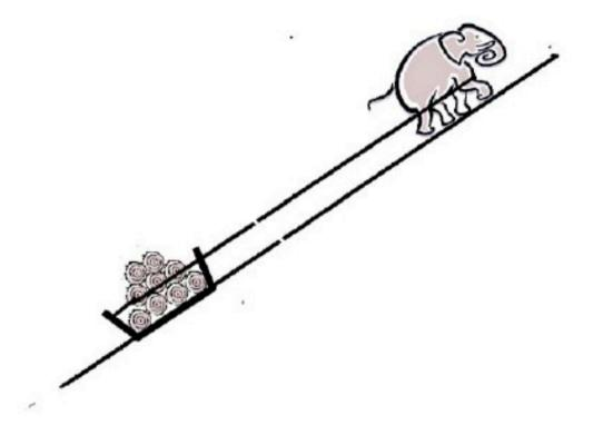
An elephant drags a tray of logs of total weight 10000 N up a uniform slope. The slope is 20 m in length and is inclined at an angle of 30° to the horizontal. The value of the coefficient of kinetic (sliding) friction between the tray of logs and the slope is 0.50. The elephant walks at a constant speed.
